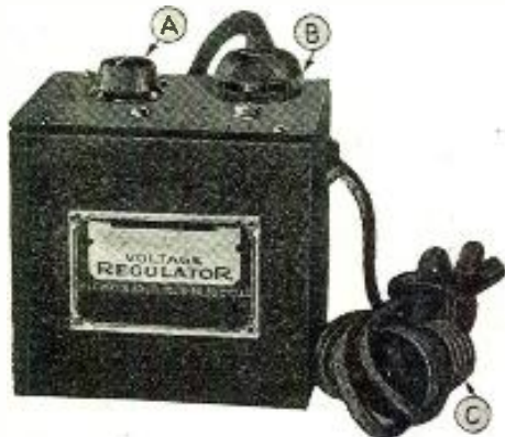
To obtain 110-volt current from a variable or non-standard lighting supply, plug the receiver's power-unit lead in at B on this device, and insert C in a light-socket. Adjustment is made by knob A, as shown in the diagram at the right.
