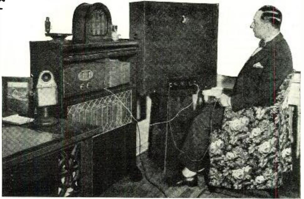
H. Gernsback, Editor of RADIO NEWS , receiving the television broadcasts from WRNY at his home in New York City, with the simple apparatus described in this article. For purposes of the test, the neon tube and loud speaker were connected in series temporarily, with successful operation simultaneously.
