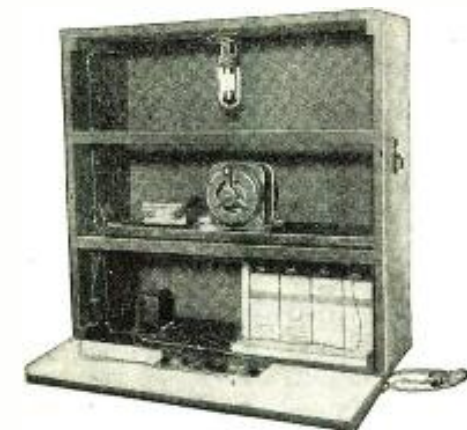
The cabinet of the reproducer with the front removed, showing the lamp and the motor with its regulating condenser. The "B" blocks are conveniently located beneath.
